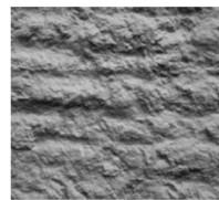
Fig. 6.9: CSP 9 (heavy scarification—rotomilled)
